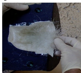
Figure 32 & 33: Laying Glass for the Part
