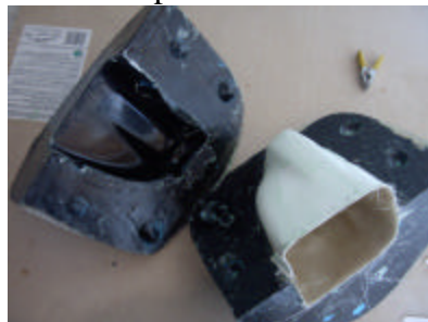
Figure 42: Part Separates From 1 st Side
