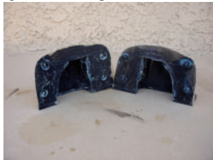
Figure 28: Completed Mold Halves
