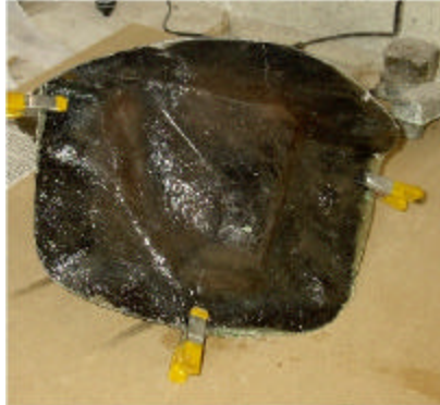
Figure 37: Mold Halves Joined
