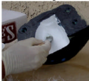
Figure 32 & 33: Laying Glass for the Part
