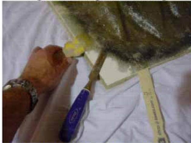
Figure 30: Lifting Mold from Plug
