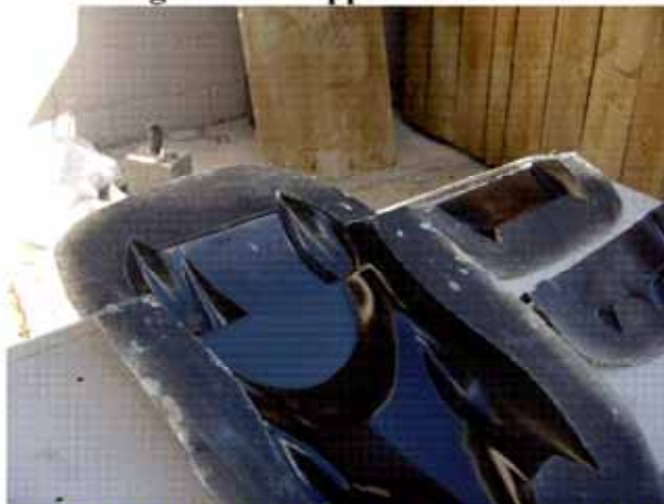
Figure 36: Prepped for Gelcoat
