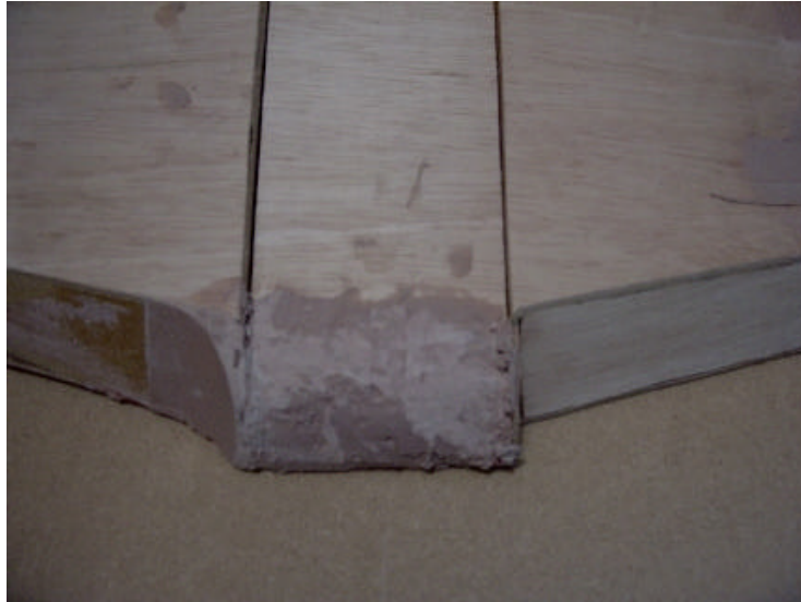
Figure 28: Shaping the Nose of The Scoop
