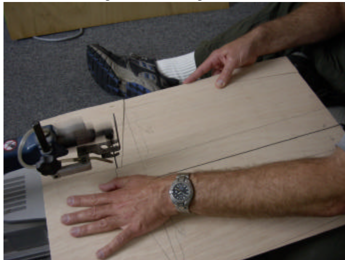
Figure 5: Cutting the Base
