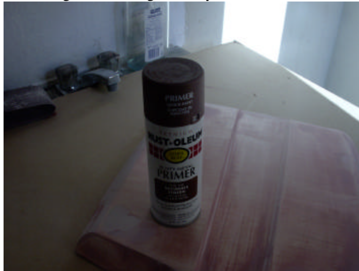
Figure 35: Plug is Ready For Guide Coat
