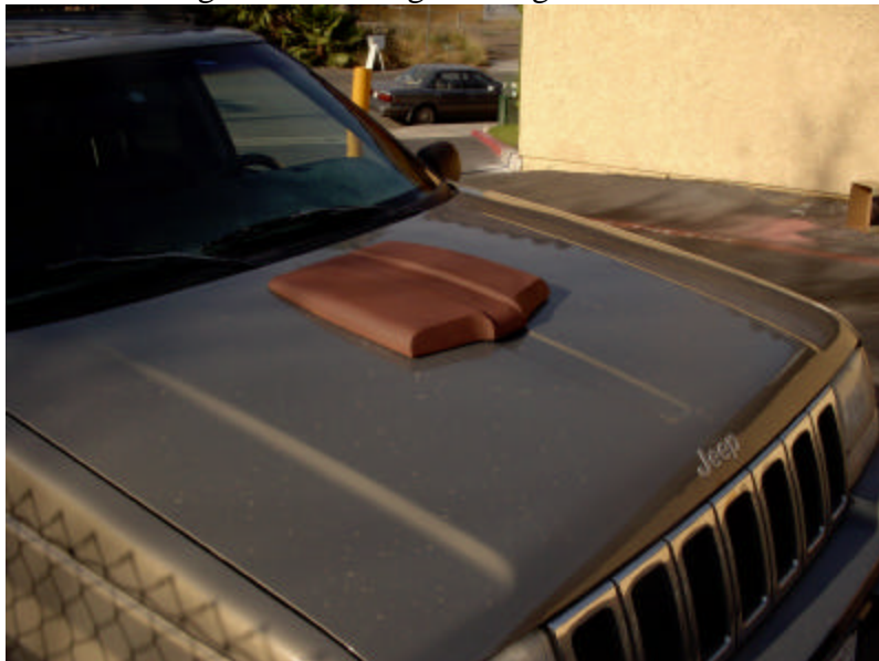
Figure 37: Fitting the Plug to the Hood
