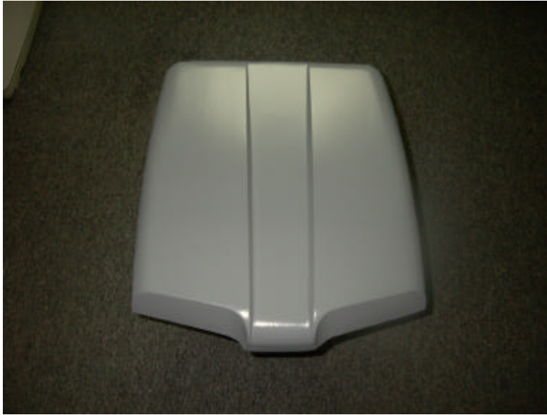
Figure 45: Plug is Ready For Molding
