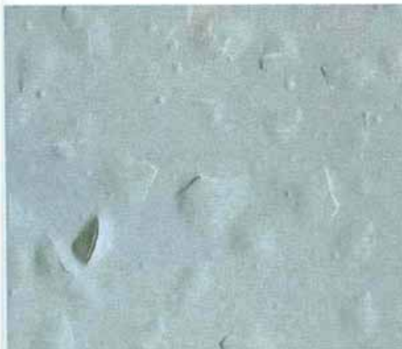
5 - Blisters - Osmotics Small blisters - gel coat; large - laminate
