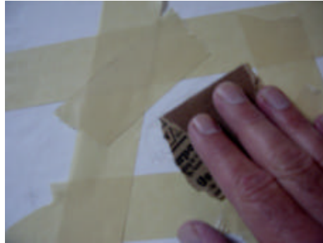
Figure 28 Sanding to Roughen the Surface
