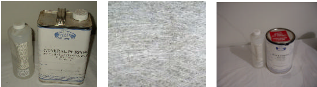
Figure 13,14 & 15 From left to right: Resin, Fiberglass Mat and Gelcoat
