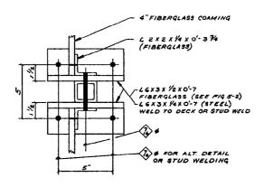
WELDED TO STEEL DECK (ALTERNATE - FAP BOLTED TO STUR A A WELDED TO FLOOR - SEE ALT DETAIL FIG 3)
