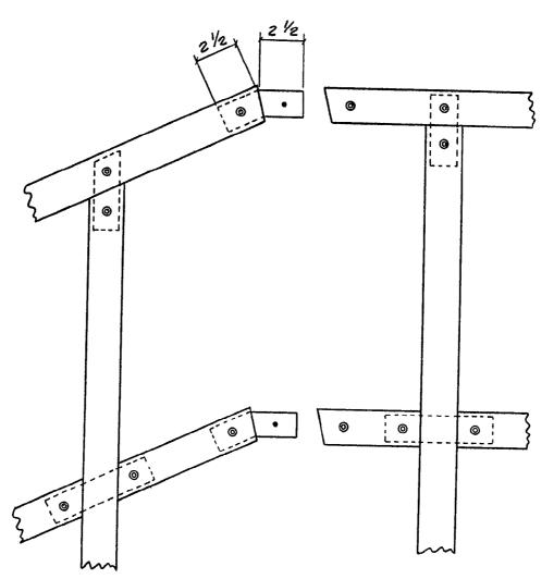
FIG. 11 Stair Rail to Rail
