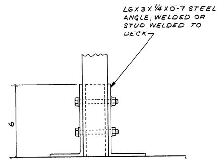
FIG. 5 Handrail Post Anchored to Steel Deck
