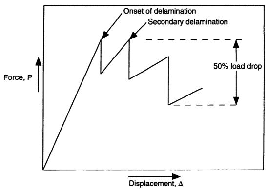
FIG. 4 Typical  $P\!/\!\Delta$  Response for a Multidirectional Specimen
