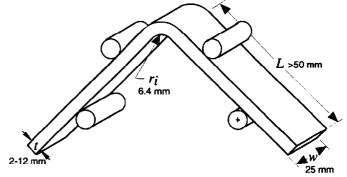
FIG. 1 Test Specimen Geometry
