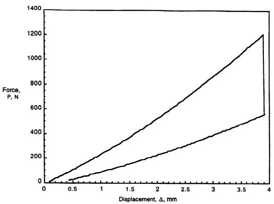
FIG. 3 Typical P/A Response for a Unidirectional Specimen
