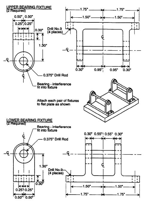
Note 1—All fillets are 3.175 mm (0.125 in.) R unless noted FIG. X1.1 Bearing Fixtures
